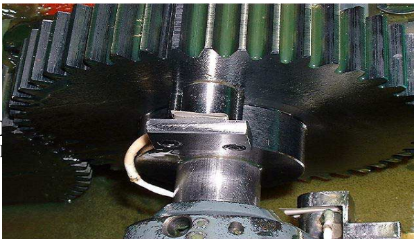
Fig.No.2 AE sensor located on pinion.
