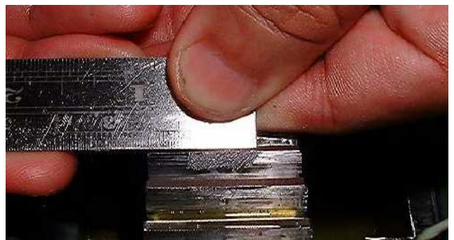
Fig.No.4 Seeded large addendum defect.
